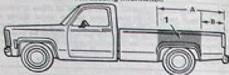
1. Recommended location for cargo center of gravity for cargo weight rating (Pickup Truck).
