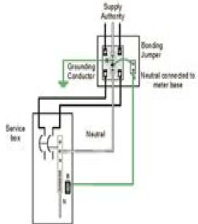
**DIAGRAM B:** Grounding at meter base
