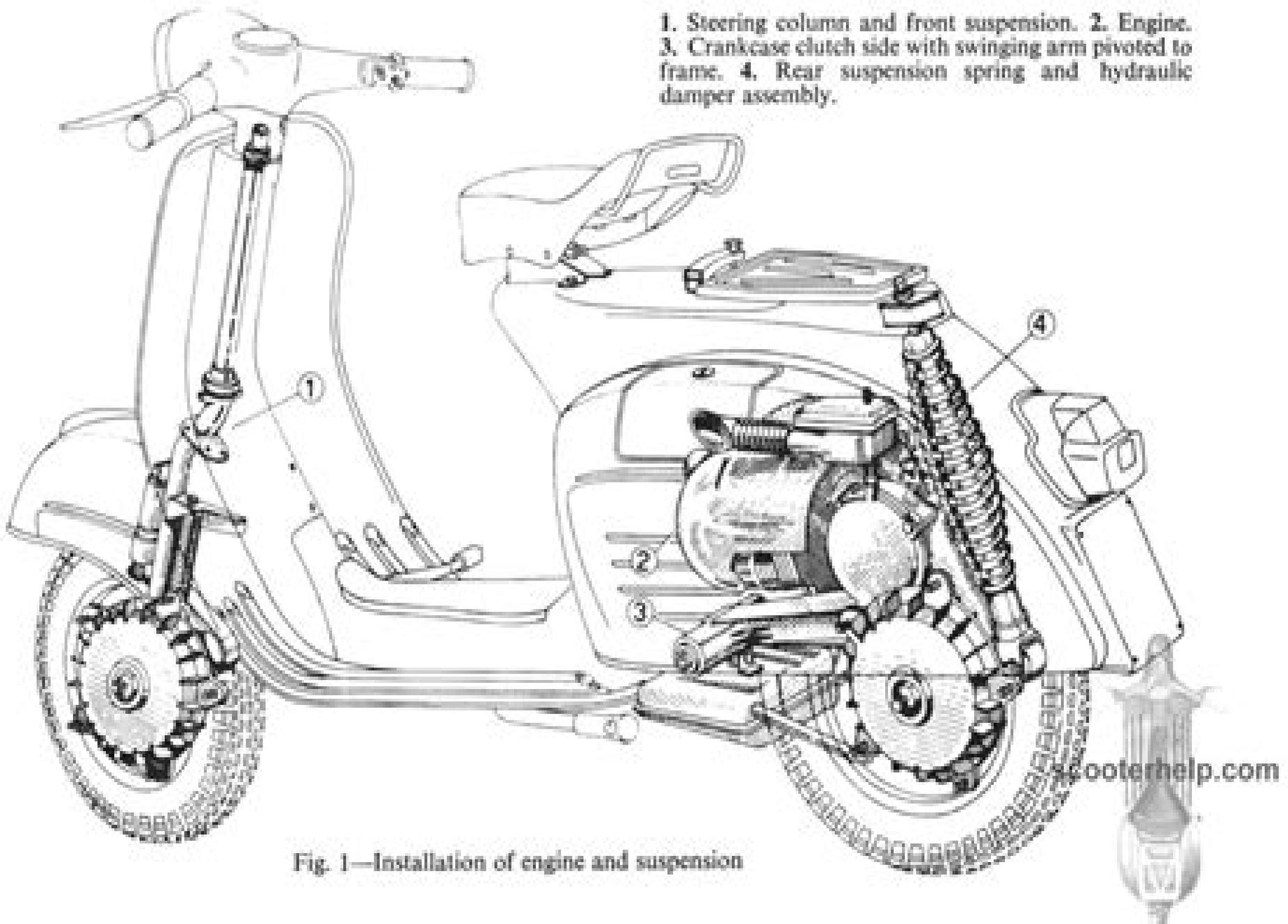
Fig. 1—Installation of engine and suspension
