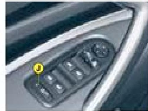
This deactivates the controls in the rear of the vehicle, both for the rear windows and for opening the rear doors from the inside. The electric child safety device is activated by pressing on button J.
