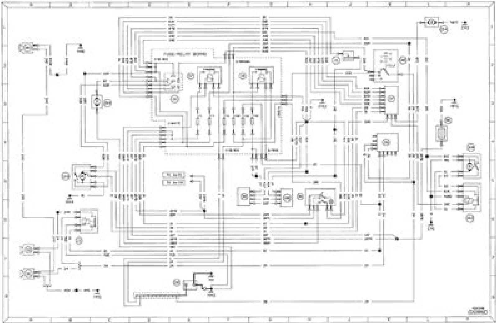
Diagram 3 : Typical auxiliary circuits (wash/wipe, horn, heater blower and heated rear window) - early models
