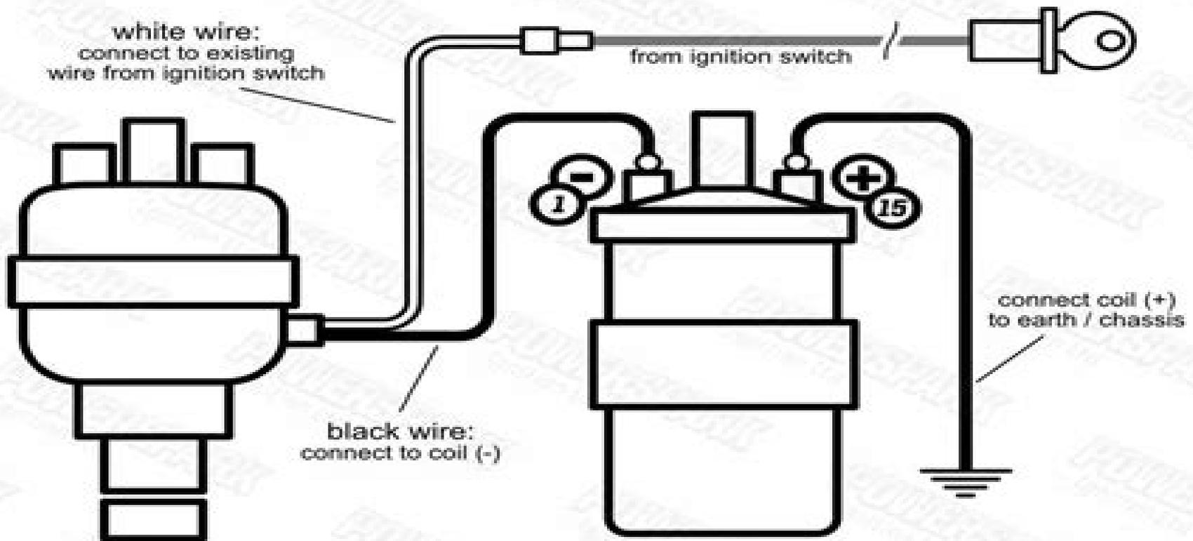
**Wiring for Positive Earth Powerspark Electronic Ignition**
